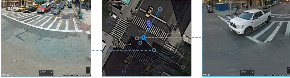
Fig. 5. In the center, the satellite image with the purple pin marking the detected crossing and the graph of surrounding street views. On the right, the closest Street View shows the crossing covered by a car. On the left, the crossing is visible.
